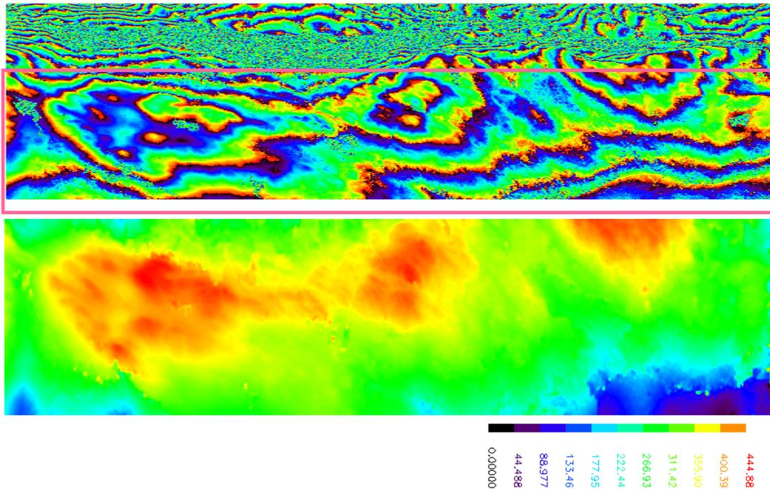
Figure 4 Digital elevation model for part of the Interferogram for Glenaffric radar data after application of filter.
