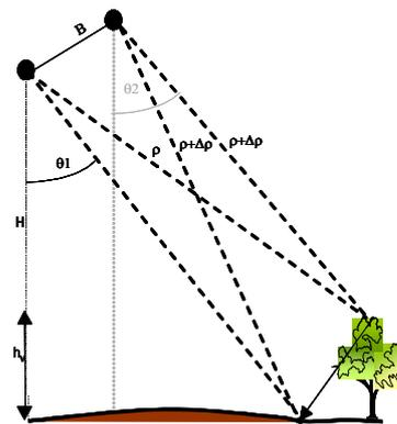
Fig (1), Schematic presentation of the scattering phase centres
