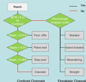
Figure 4. Channel typing schema. Reaches less than 8 m bankfull width were classified into 4 confined channel types based on Montgomery & Buffington (1977). Reaches with bankfull width > 8 m and unconfined were classified as migrating (Hall *et al.* 2007) and subjected to further classification with LDA.
