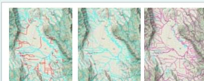
Figure 3. Historic channel reconstruction processes. Artificial channels (red lines) were removed, and isolated streams were reconnected with a minimum amount of artificial channels.
