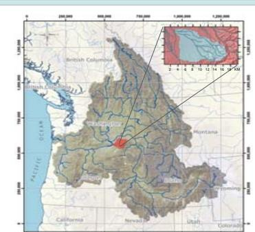
Figure 2. The Columbia River basin and the scale of channel typing. The total length of reaches in the GIS layer is 444,121,266 m and the number of reaches are 2,273,010. A blue area in the Walla Walla watershed (red area) includes 295 reaches, all of which are 200 m long.
