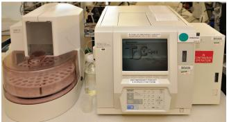
**Discrete Analyser** This versatile instrument can analyse a wide range of parameters, such as the phosphate and ammonium content.
