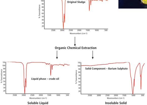
Comparison of the Infrared Spectra of the two fractions shows that the sludge is a mixture of Crude Oil and Barium Sulphate (drilling mud component)
