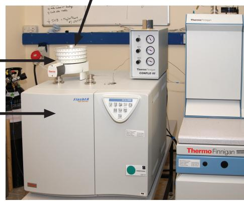
Inside the elemental analyser the soil is burnt at 1020°C in a burst of oxygen. All the carbon in the soil is converted to carbon dioxide which is carried to a mass spectrometer where it is measured.
