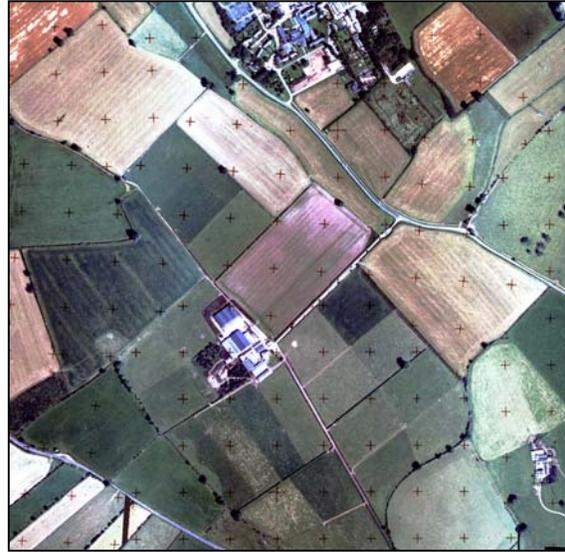
Figure 2. Orthorectified and mosaiced colour photography 1:5000
