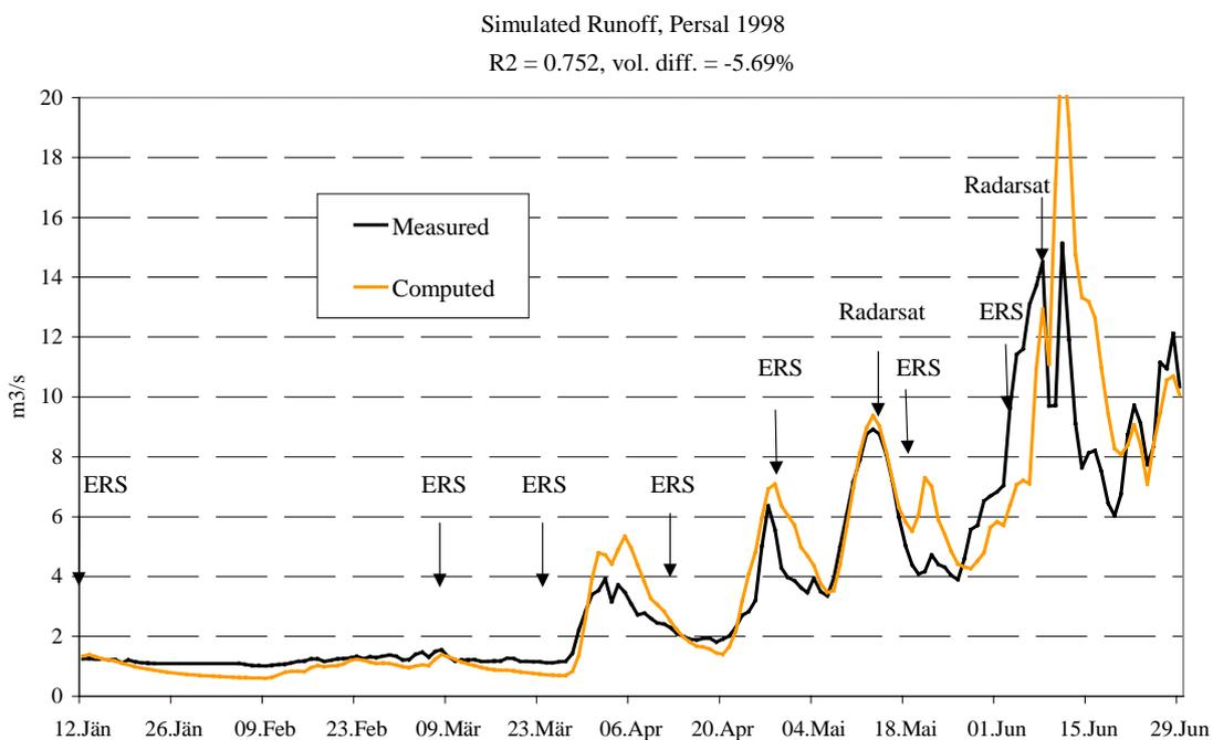
**Figure 6:** Measured and simulated runoff for the basin Tuxbach in spring 1998. The arrows indicate the acquisition of SAR images used for the model calculation.
