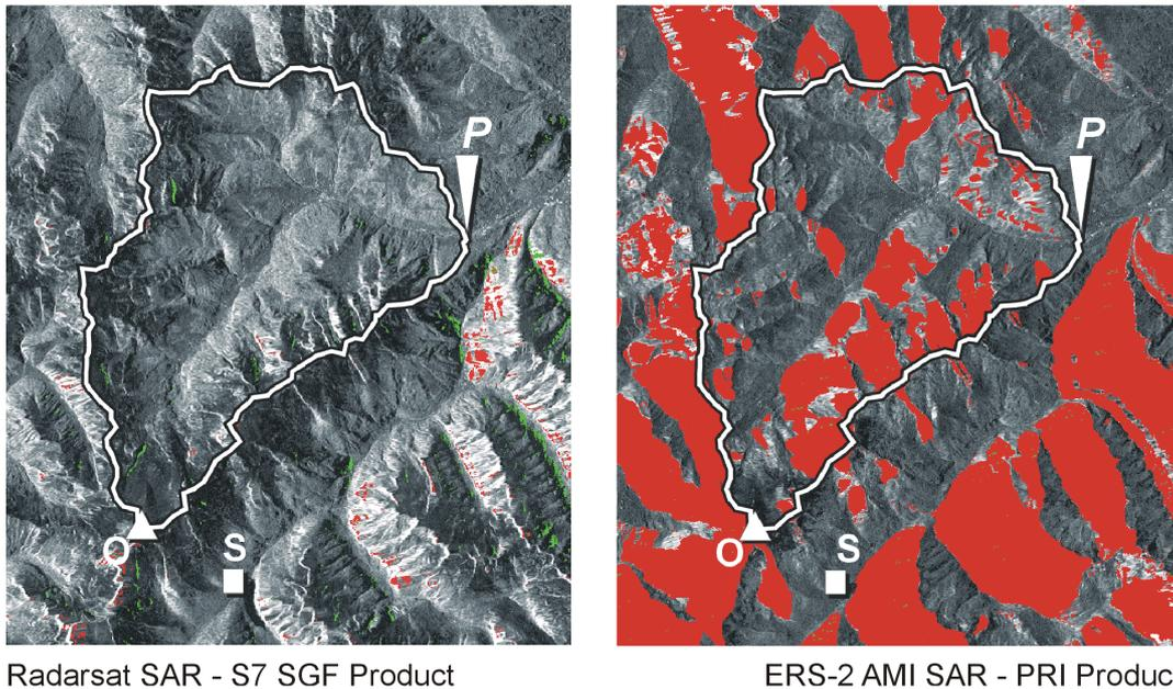
**Figure 3:** Geocoded Radarsat SAR Mode S7 image, 13 May 1998, (left) and ERS-2 SAR image, 6 July 1998, (right). Layover regions (red), radar shadow (green).
