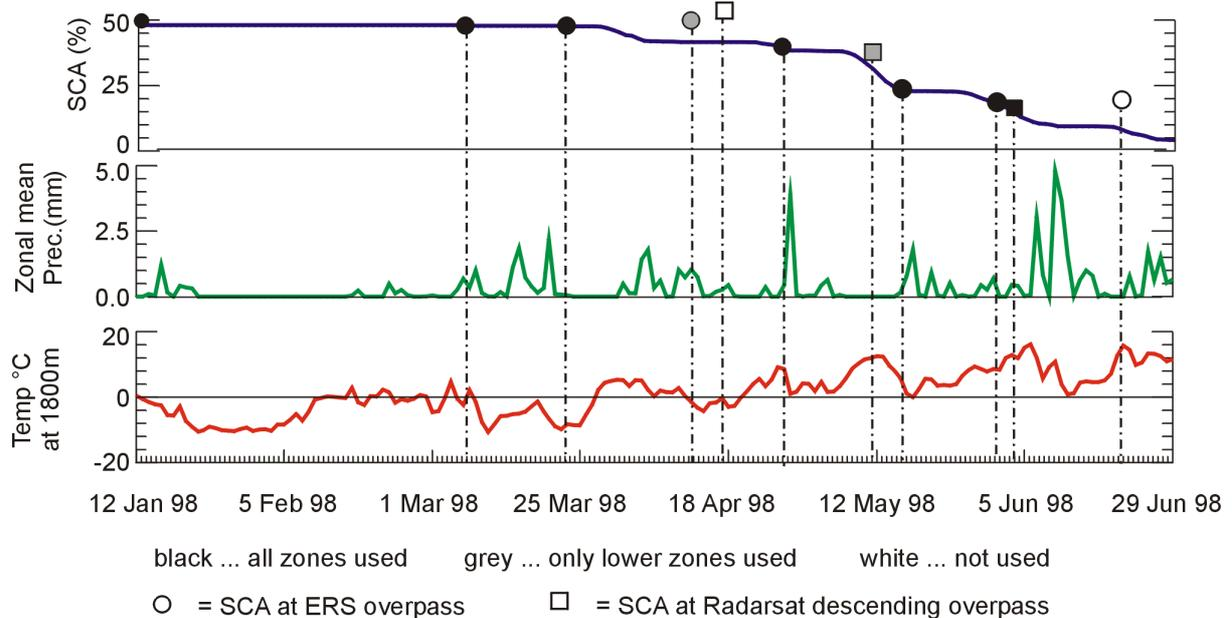
**Figure 5:** Daily values of the snow covered area (SCA) in the basin Tuxbach / Zillertal derived from ERS-2 and Radarsat SAR data, the mean zonal precipitation and the typical temperature at 1800 m based on daily measurements at the stations Schlegeis and Mayrhofen.
