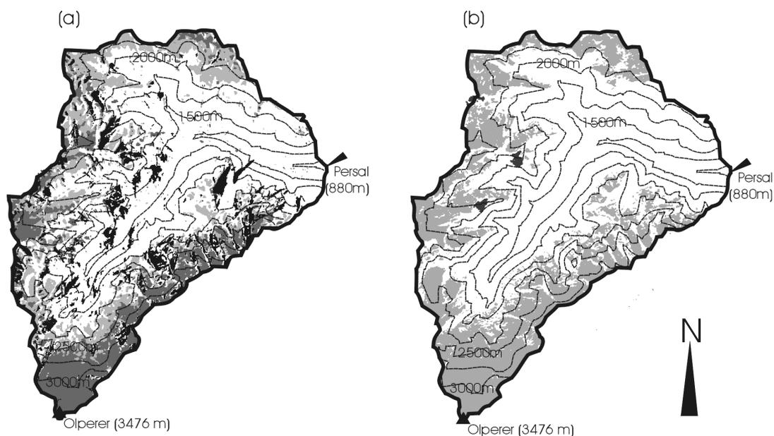
**Figure 4:** Snow map from (a) Radarsat SAR data beam mode S7; light grey: change of snow extent between 11 May 1998 and 4 June 1998, dark grey: snow extent on 4 June 1998; and (b) from Landsat-5 TM data 13 May 1998; light grey: snow; black: no information (clouds in Landsat TM image; SAR: layover, radar shadow, and local incidence angles  $<17^\circ$  and  $>78^\circ$ ); white: snow free areas.
