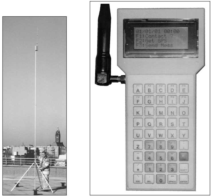
Figure 3: Autonomous (left) and mobile handheld groundstation (right)
