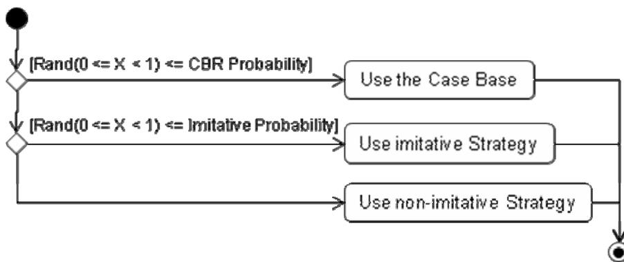
**Figure 11** — UML Activity Diagram showing part of the decision-making algorithm of Land Managers of the CBRStrategyLandManager class. This algorithm replaces the 'Choose a Land Use for the Parcel using the Case Base' steps in the algorithm shown in Figure 10 for the CBRSocialParcelLandManager class.
