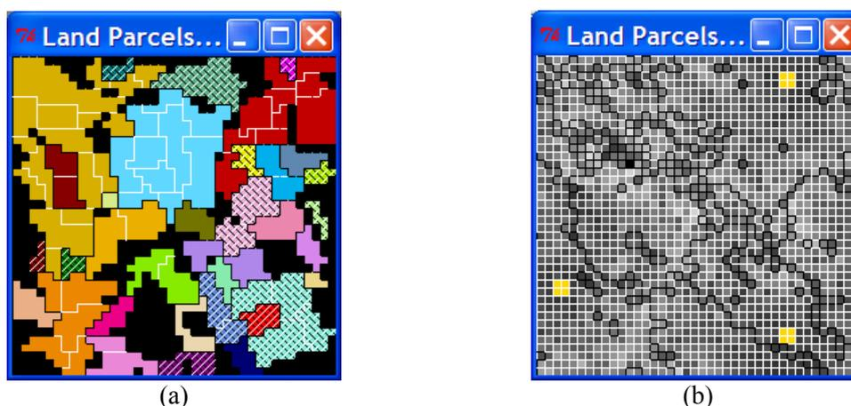
**Figure 38** — (a) showManagerRaster = 1. A black boundary is drawn between Parcels owned by different Land Managers, and a white boundary between Cells belonging to different Parcels. Diagonal black and white lines through the Cells indicate a bankruptcy. (b) showManagerChangeRaster = 1. (Not from the same model run as (a).) Lighter shades of grey indicate more changes of Land Manager. Yellow Parcels indicate no change of Manager.
